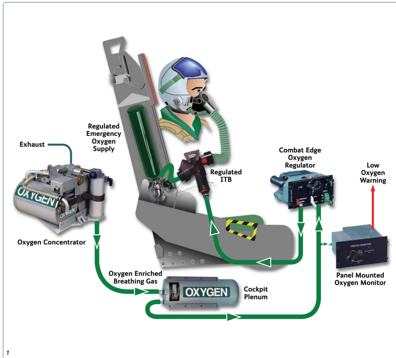
Cobham has established the installation of its flight-proven On-Board Oxygen Generating System (OBOGS) on the Lockheed Martin F-16 Falcon aircraft to replace the liquid oxygen system (LOX). Minimal modification is required to retrofit the aircraft with OBOGS.
