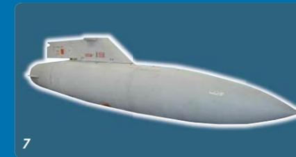
7 **External Aircraft Fuel Tanks:** Cobham designs and manufactures fuselage, centerline and wing tanks
