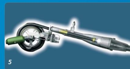
5 **Air-to-Air Refueling Hose Drum Units:** Extendable and retractable, the hose drum units provides probe and drogue refueling
