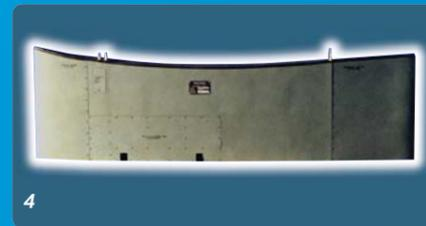
4 **Universal Pylon:** Cobham's C-130 Universal Pylon enables weapons or special purpose pod integration
