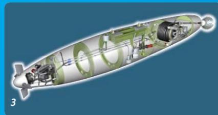
3 **Air-to-Air Refueling Pods:** Wing tip and Buddy Store aerial refueling pods are self powered by a Ram Air Turbine
