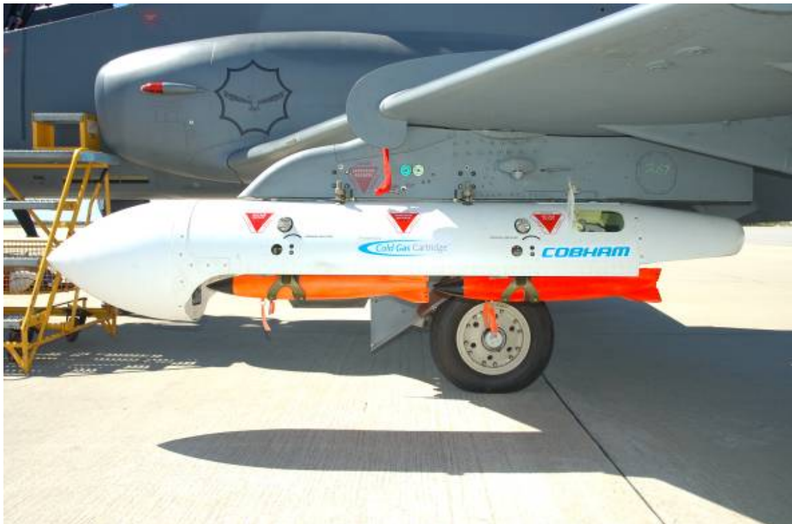
A South African Air Force Hawk light attack aircraft equipped with a Cobham Carrier Bomb Light Stores (CBLs) ejector rack with four 12.5kg practice bombs ready to be dropped using Cobham's Cold Gas Cartridge.
