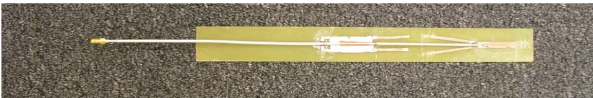
Figure-7: Dipole Antenna
