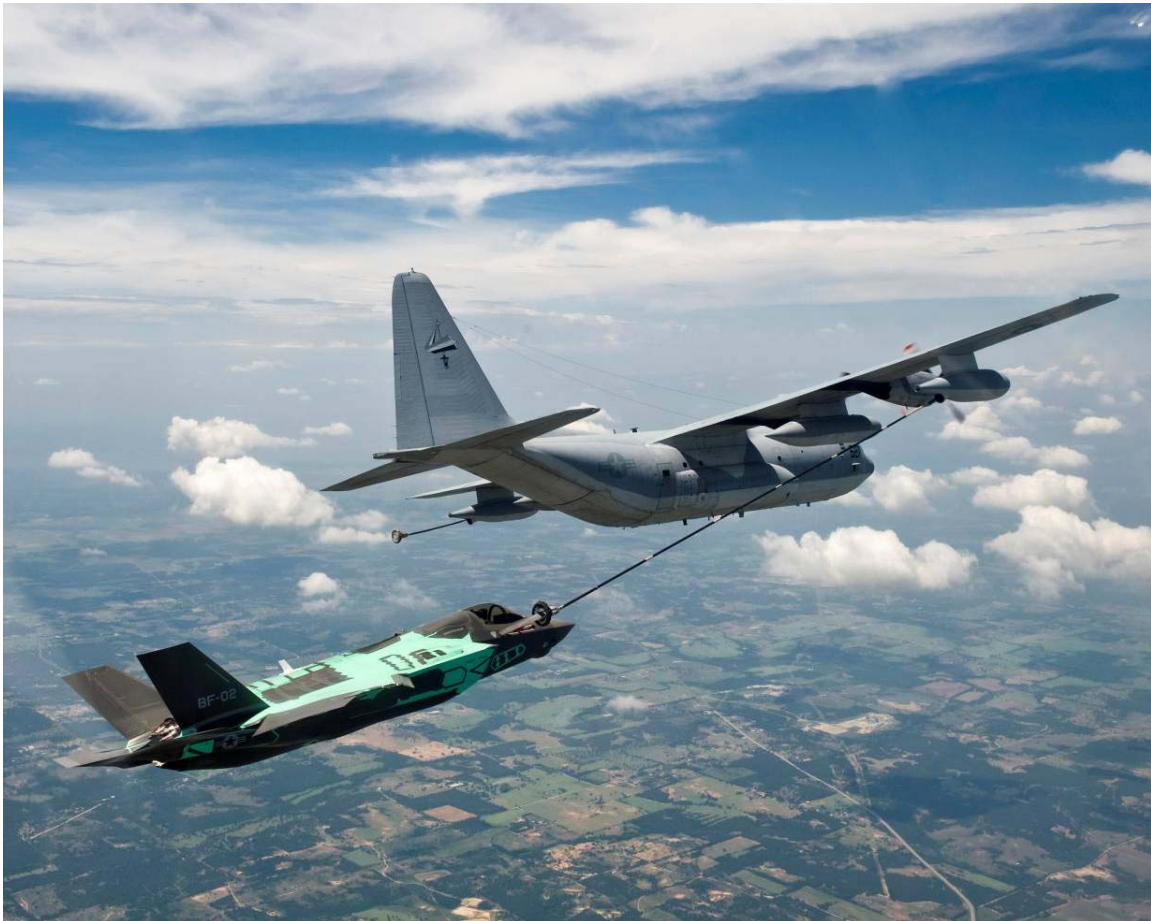
Image caption: A USMC KC-130 tanker equipped with Cobham aerial refueling pods passes fuel to an F-35B STOVL variant equipped with a Cobham aerial refueling probe during recent tests over Texas; image courtesy of Lockheed Martin.
