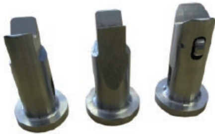
Pawl Enhancement (left to right) original, worn and new design
