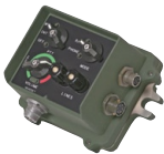
Infantry Telephone Station (ITS/R). Provides external infantry personnel with access to the intercom and CNR on the platform.
