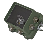
Master Control Station Light (MCS/L). The MCS/L provides similar functionality as the MCS in a small footprint.
