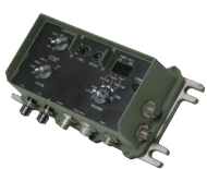
The Master Control Station (MCS). This provides central power and system control. Incorporates BIT and programmable control over user access to external radios.
