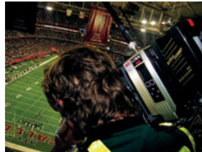
The AVS/LinkHD RF system debuted successfully at a Monday Night Football game in December, with the LinkHD transmitter and a battery block attached to a Thomson LDK 6000 camera
