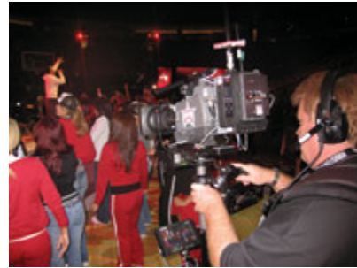
TNT used LinkHD RF technology during pre-game and halftime shows at the NBA All-Star Game, this time configured for Steadicam and transmitting to the receiver/decoder in a production truck outside.
